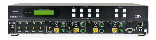
The KanexPro MX-HDBASE4X4-4K matrix switcher is a professional 4 HDMI input to 4HDBaseT output switch with 2 HDMI mirrored outputs designed for routing 4K/UHD applications. For proficient audio capabilities it includes 4 auxiliary audio input for stereo and audio de-embedding using digital coax. Supporting HDMI High Speed Specifications featuring data rates up to 10.2 Gbps, Deep Color up to 16-bit, 3D, Lip Sync, and HD lossless audio formats.
